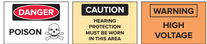
Figure 1-5 Typical safety signs.
